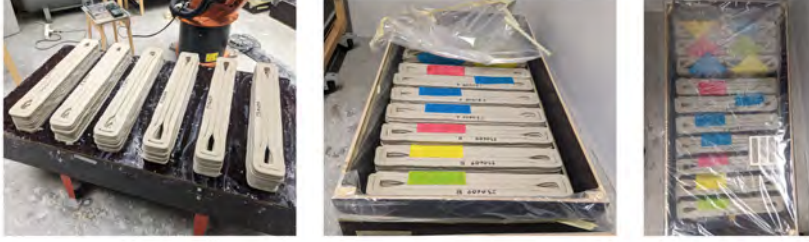
Figure 5.8: Controlled humidity curing chamber.
