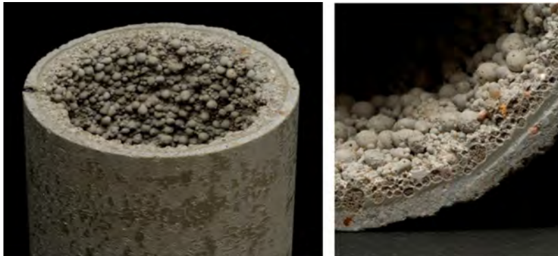
Figure 3 – An example of controlled segregation by rotating the fresh mix on a lathe. Reproduced from [45]
