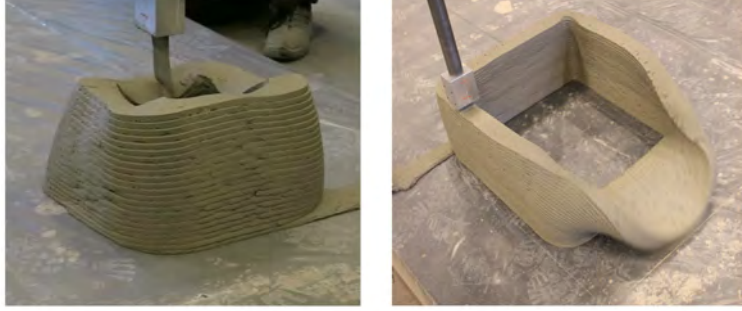
Figure 2.18: Main failure modes in 3D Concrete Printing (3DCP). Left: Plastic yielding due to insufficient yield stress (material failure). Right: Elastic buckling due to insufficient stiffness (stability failure). Reproduced from [53].
