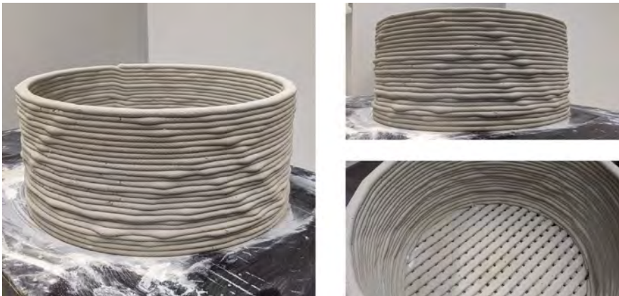
Figure 6. Printed prototype showing the projected image as variable wall thickness. Variations in printing speed are combined with a compensation algorithm to restrict the effect of the variation to the outer face of the printed part.
