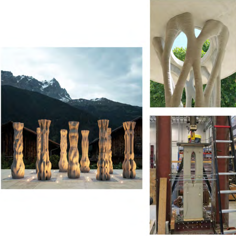
Figure 2.12: Some examples of 3DCP columns. Left: Truss-shaped pillar by XtreeE [99], Centre: Prefabricated columns printed at ETH Zürich [100], Topology optimised column prototype testing [97]
