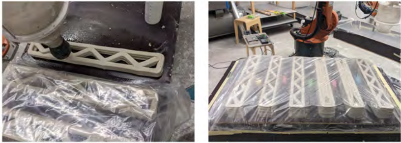
Figure 5.7: Covering the printing specimens to avoid excessive shrinkage due to water loss
