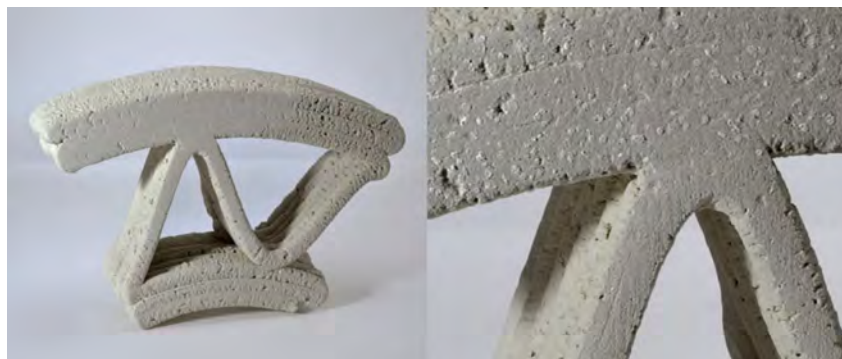
Figure 4 – Functionally graded 3D printed concrete by variable addition of lightweight fillers within higher ratios of insulating material away from the centre. Reproduced from [62]
